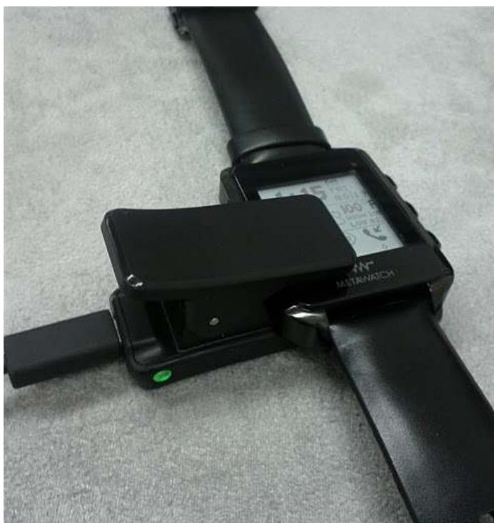
Connect the clip to the watch, plug in the USB cable (a micro USB cable is supplied in the box for you) and plug the other end into a USB power supply. When the clip has power, the clip's LED will turn on. The watch is designed to recharge from this micro USB port and also operate while charging.
