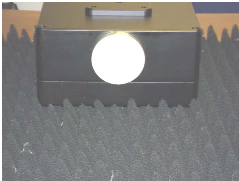
Transmitter front view (upside down) showing antenna lens
