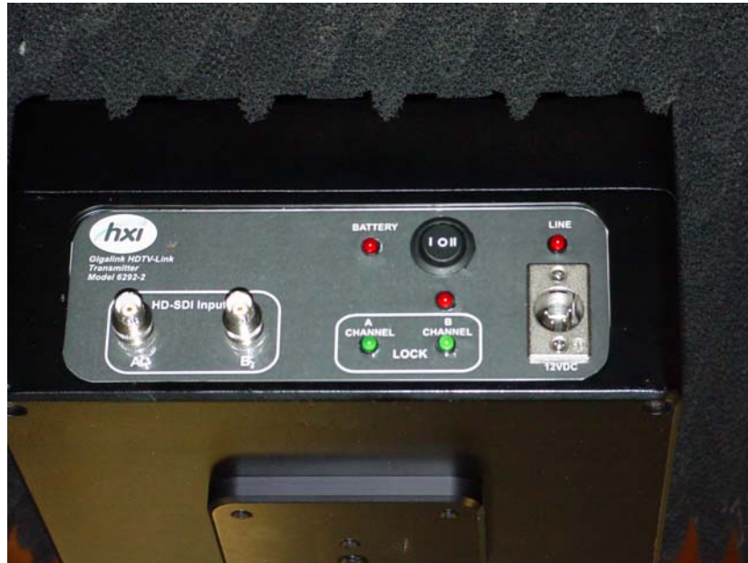
Transmitter rear view showing interfaces
