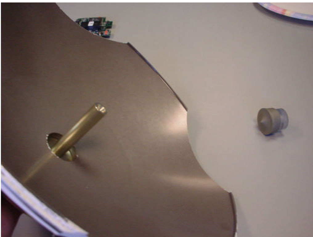
Disassembled 40dBi Parabolic Antenna with Radome mounted Sub-reflector
