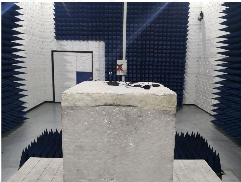
RADIATED EMISSION TEST SETUP ABOVE 1GHZ
