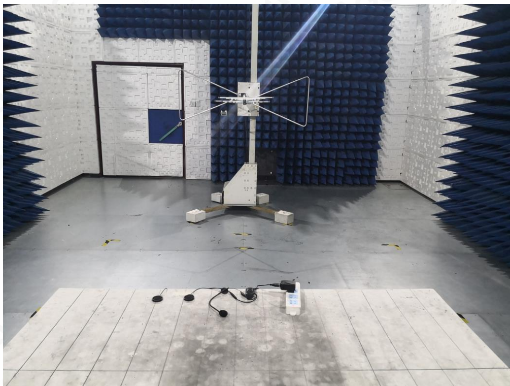
RADIATED EMISSION TEST SETUP ABOVE 1GHZ
