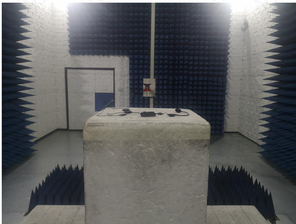
RADIATED EMISSION TEST SETUP ABOVE 1GHZ
