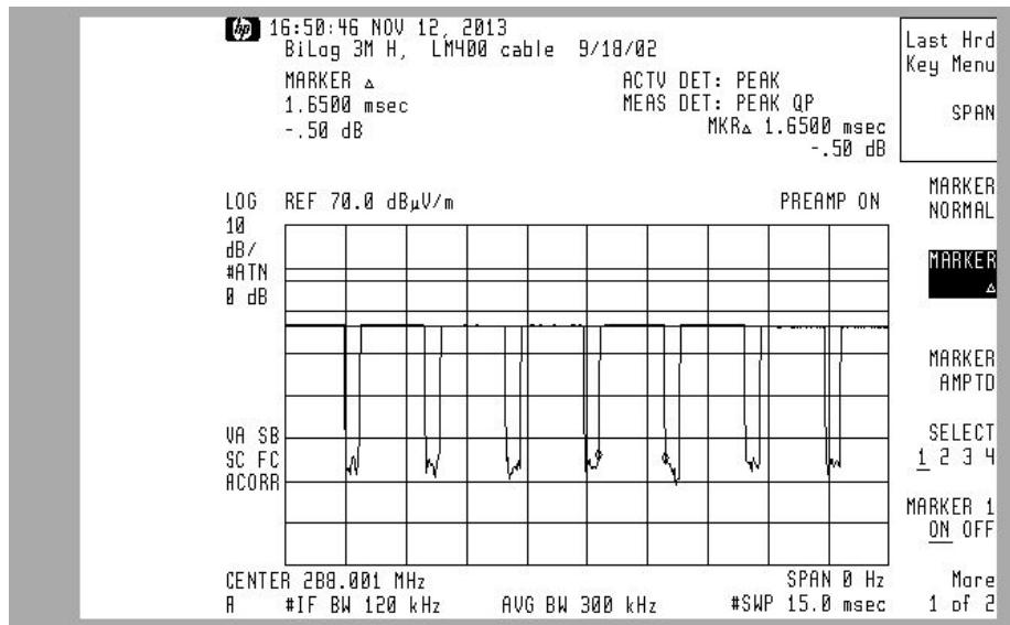
**20 dB Bandwidth Measurement:****Tabulated Summary of 20dB Bandwidth Measurements**
