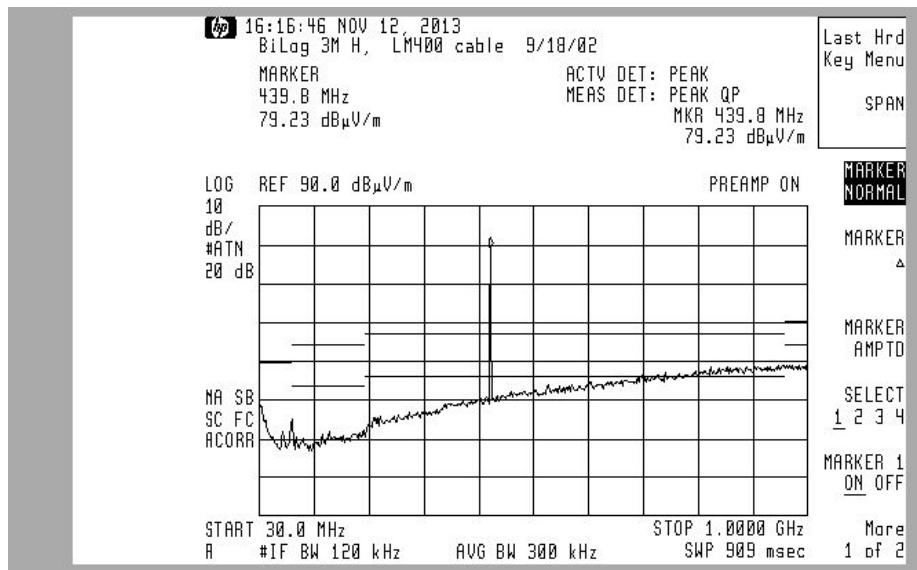
Note that marker frequency is inaccurate due to broad span of scan.
