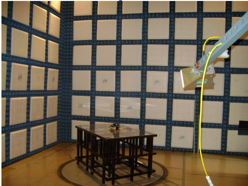
Test Set-up for Radiated Emissions, 1GHz to 5GHz – Vertical Polarization
