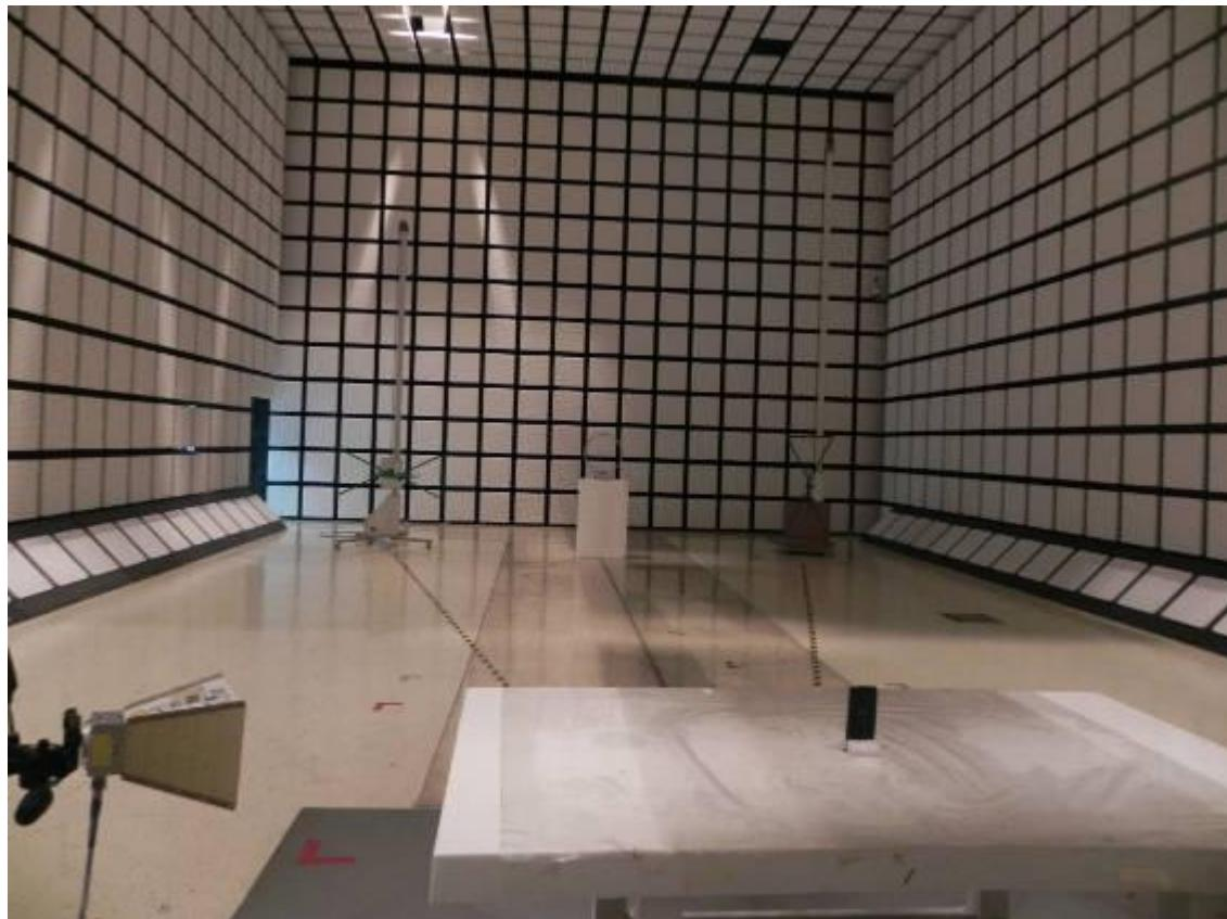
Description: Radiated Spurious Measurement Setup (From 30MHz to 1GHz)
