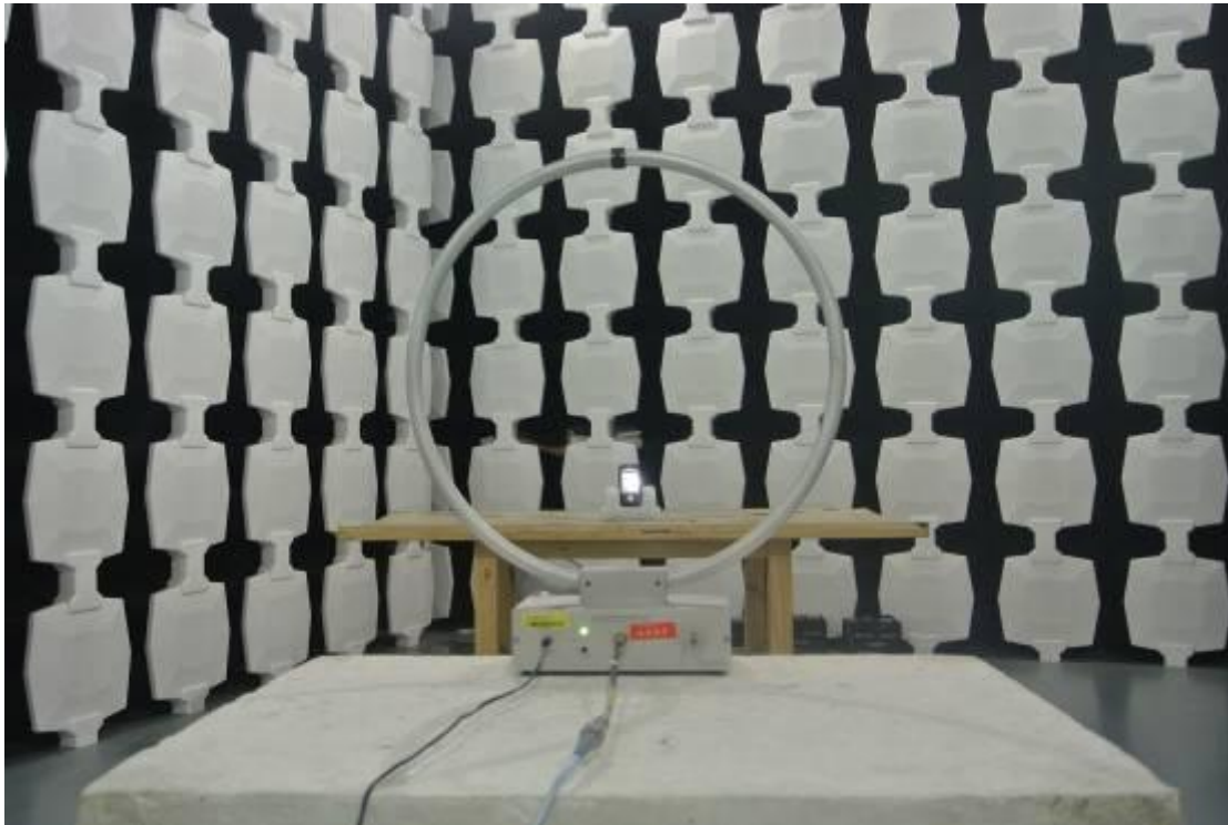
Radiated Spurious Measurement(below 30MHz) Setup
