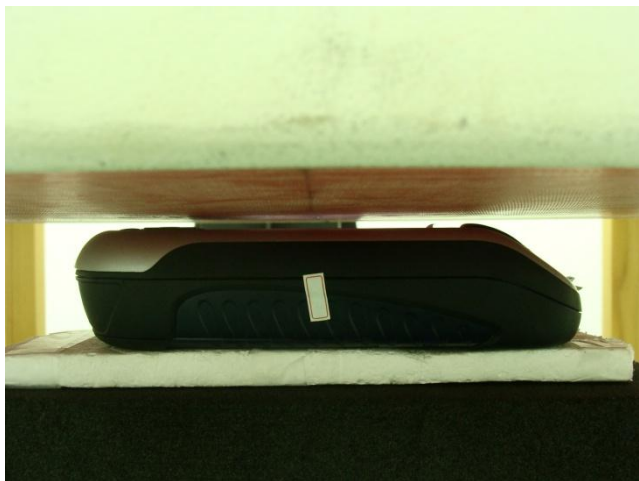
Face of the DUT with Phantom 0.5 cm Gap
