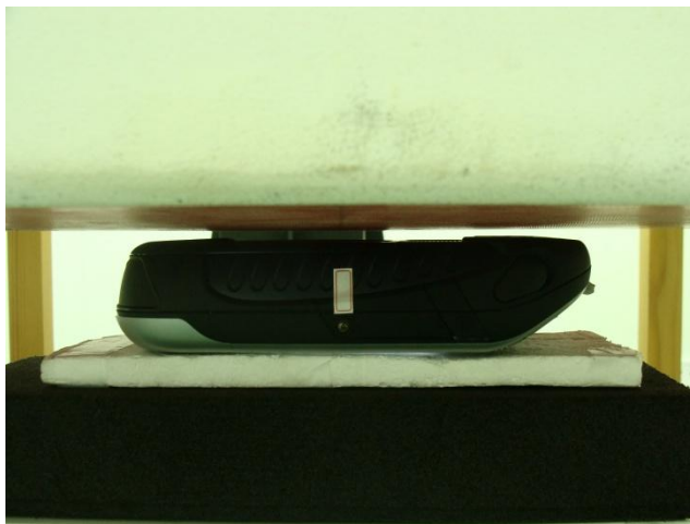
Bottom of the DUT with Phantom 0.5 cm Gap
