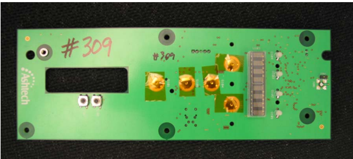
Circuit Board (Front Panel Circuit Board with BlueTooth Transceiver) Rear Side – antenna disconnected
