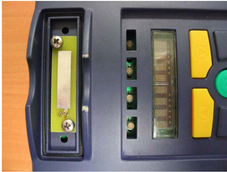
Close up view showing the BlueTooth transceiver's antenna behind a plastic bezel in the front panel (above) and the location of the front panel board in the system (below)
