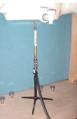
1900MHz Dipole Setup
