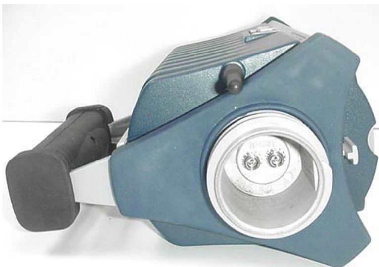
Top end of Z-Max.Net with GPS Antenna Removed (SAR test configuration)
