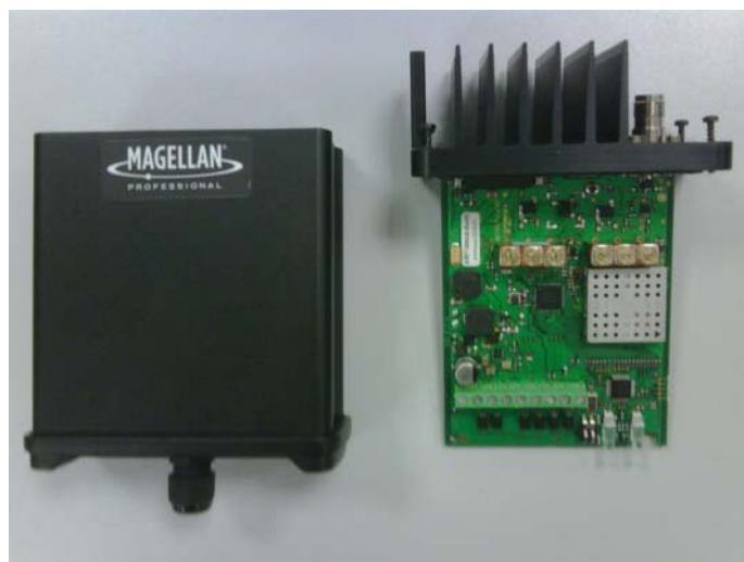
The U-Link TRx must be supplied from a DC voltage source. The input DC power voltage range is 9V up to 28V, and the total power consumption is less than 1.5A under 12V at full RF power with an antenna connected on the RF port output.
