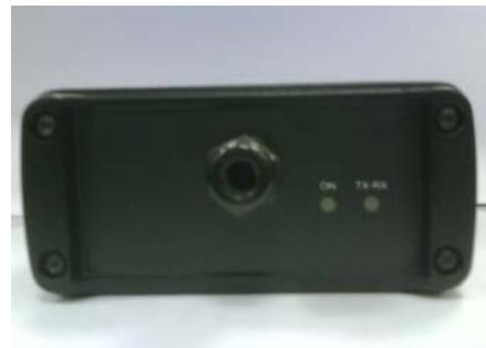
A light continuously on when the transceiver is powered on. The color of this light is changed according to the selected serial link mode (RS232 → Green, or RS422 → Red). Corresponding marking of the light shall indicate "ON"
