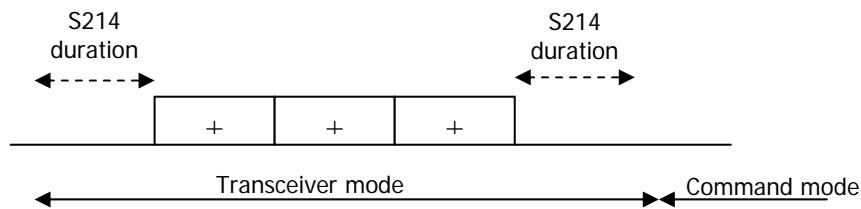
**Exiting command mode** (return into normal mode): send the serial command ATO<cr>
