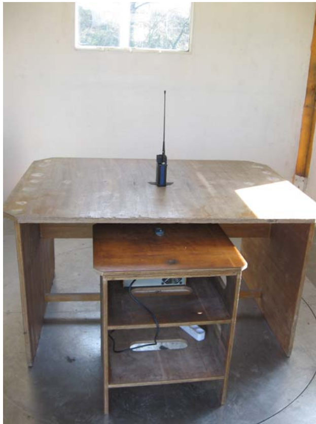
Test set up radiated measurement with antenna
