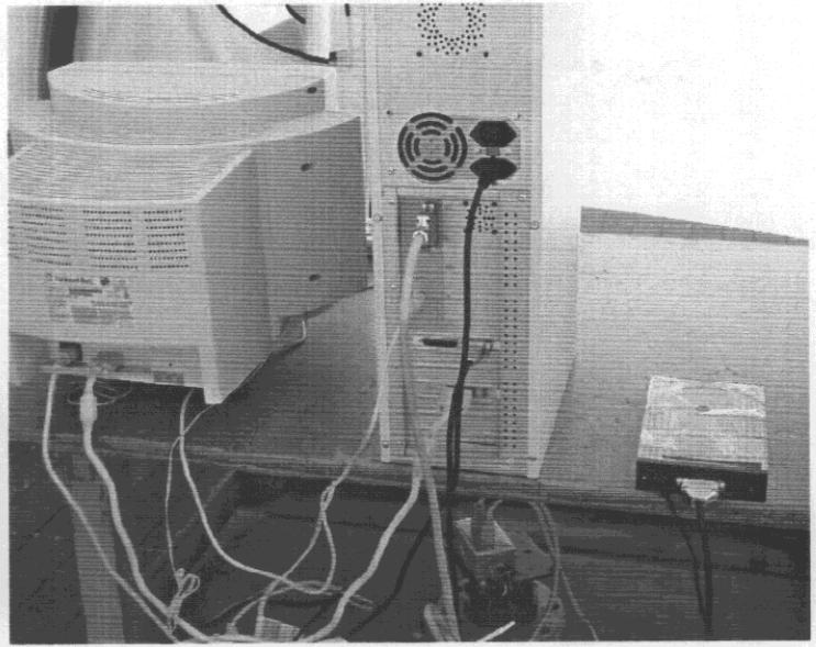
Radiated Emission Setup Photos (Worst Emission Position)
