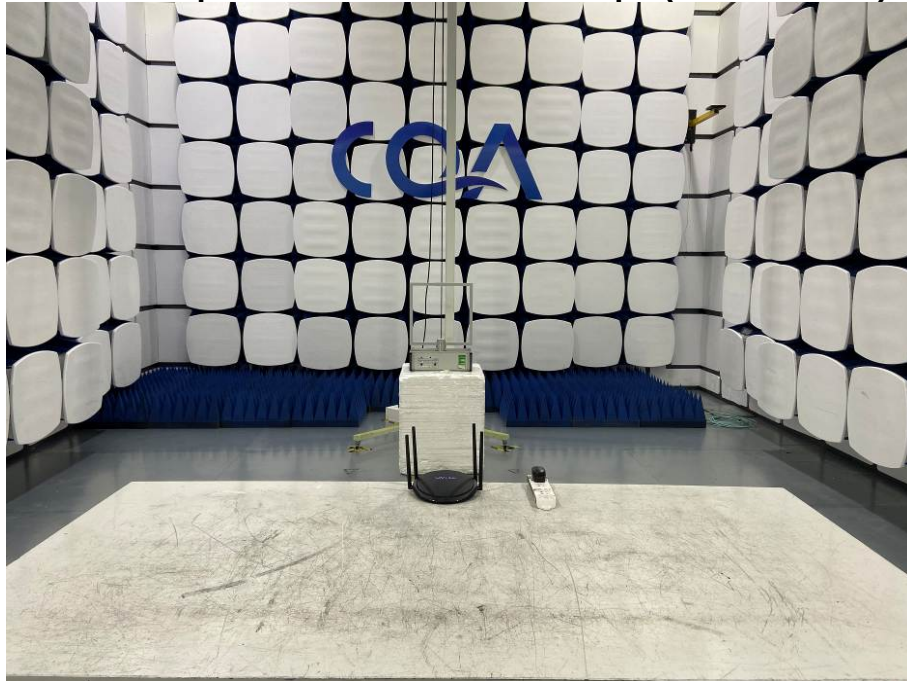
Radiated spurious emission Test Setup-1(Below 30MHz)
