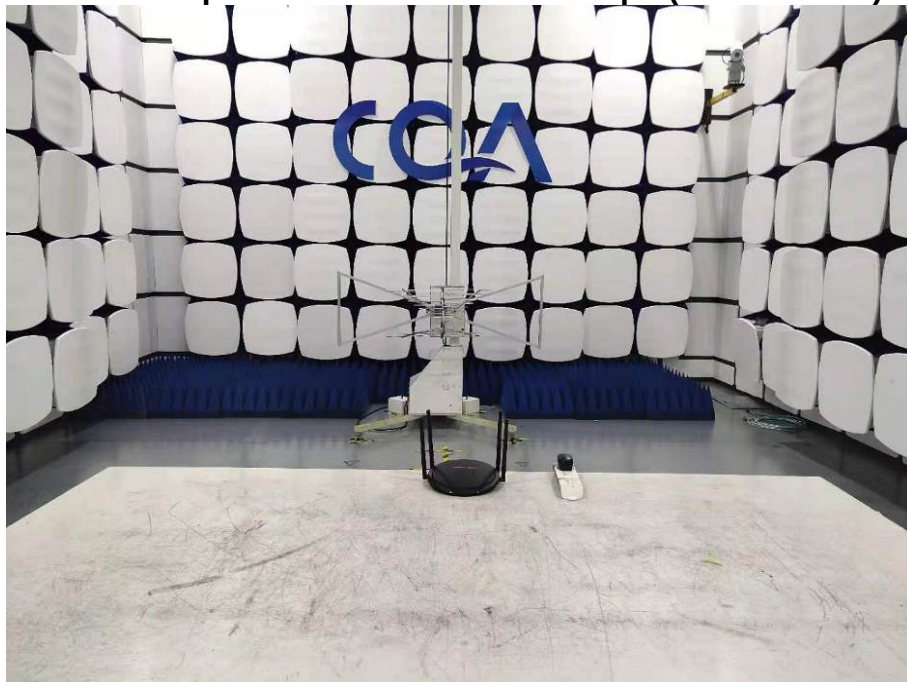
Radiated spurious emission Test Setup-2(30MHz-1GHz)
