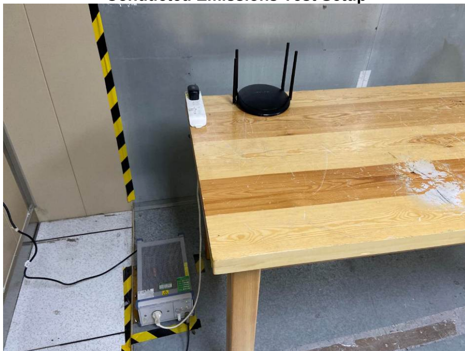
Conducted Emissions Test Setup
