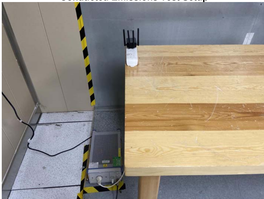
Conducted Emissions Test Setup
