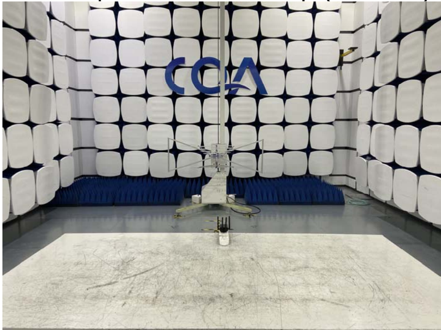
Radiated spurious emission Test Setup-2(30MHz-1GHz)
