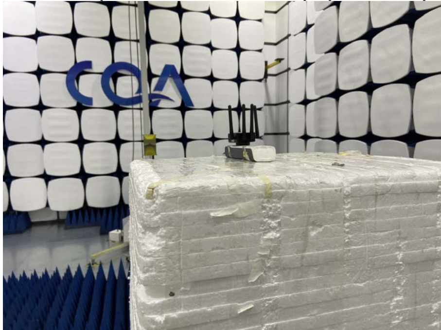
Radiated spurious emission Test Setup-3(Above 1GHz)
