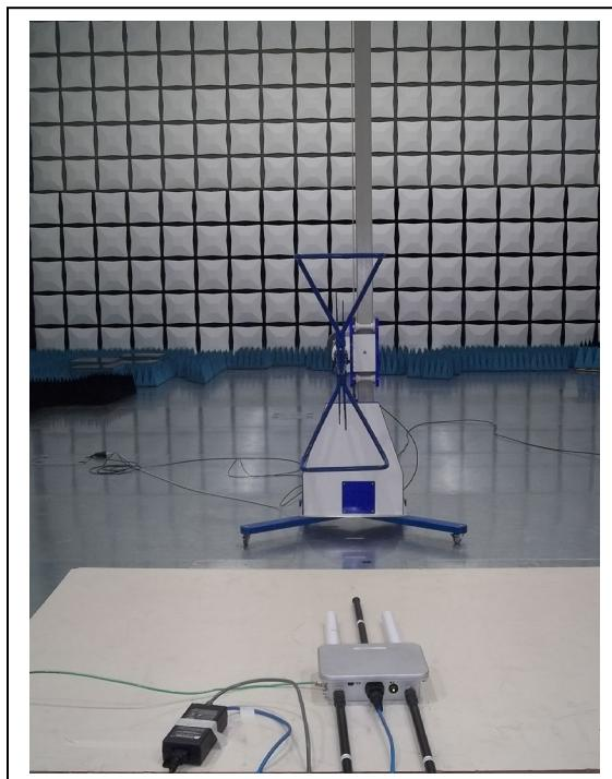
**Radiated Spurious Emissions: Greater Than 1 GHz**
