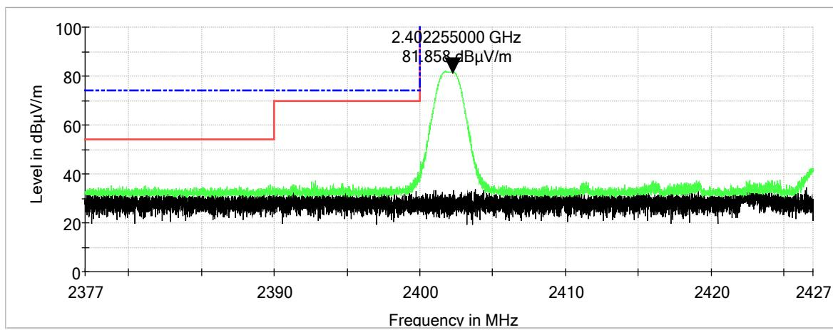
**Band Edge: High Channel, Vertical**
