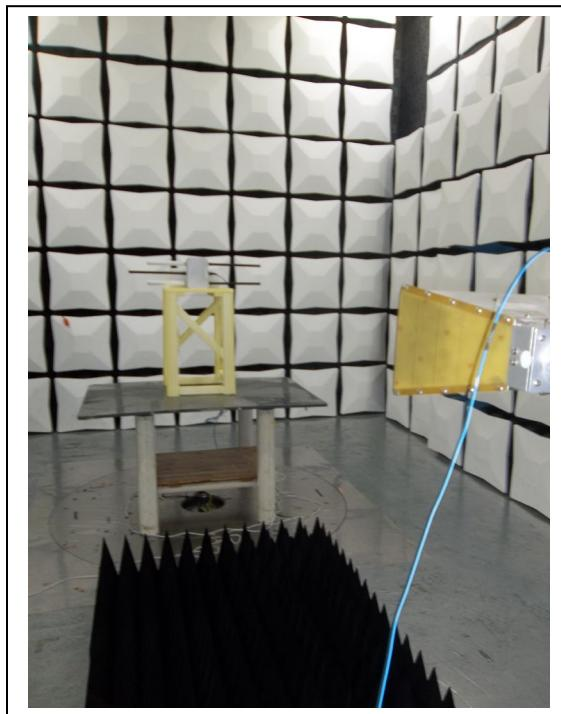
**Conducted Output Power, Peak Power Spectral Density, Occupied Bandwidth, and Conducted Spurious Emissions**
