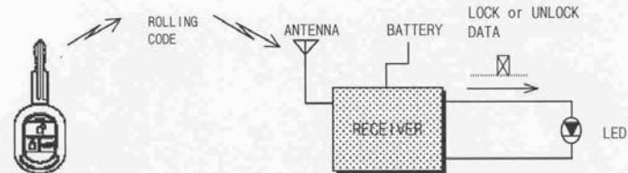
\* Through use of the LED, operating state is displayed by LED.
