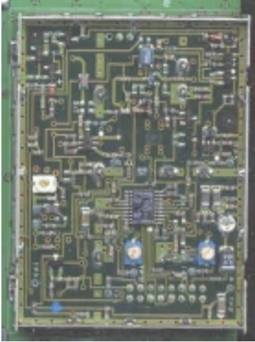
Photo 7. EUT, Top View of Transceiver Board (Shield Removed)
