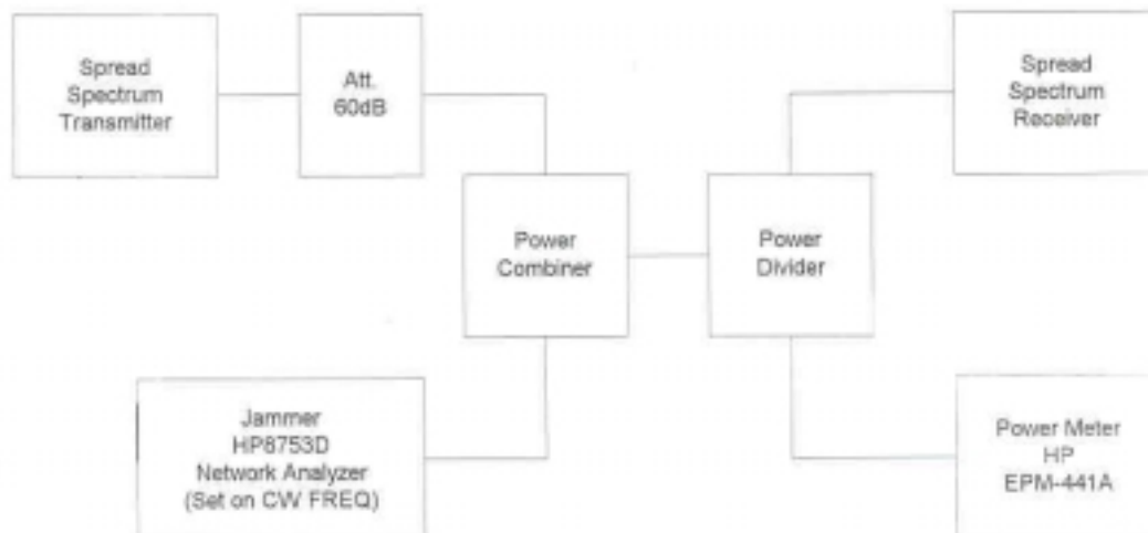
Figure 1.Processing Gain Measurement Setup
