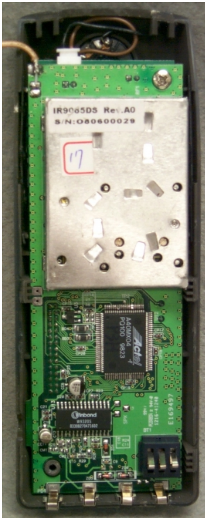
Photo 6. EUT, Top Side of Main Board
