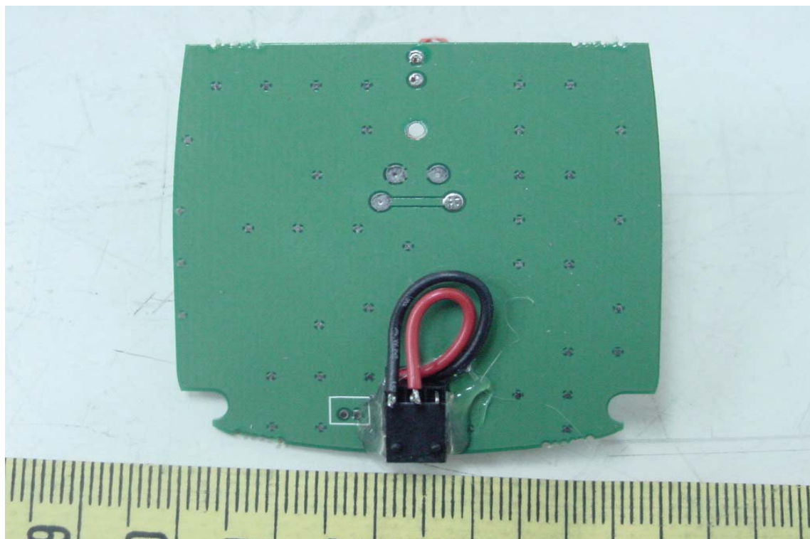
Solder View of Main PCB (Charger)
