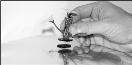
Fig. 4 - It is pretty simple to attach the Microblimp Gondola to the balloon with the supplied velcro or you can even use cellophane tape
