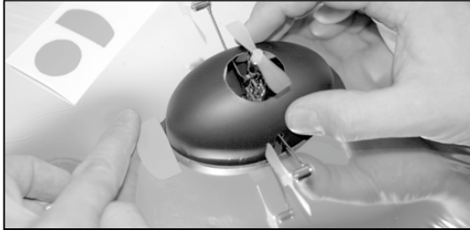
Fig. 7 - Finish off the gondola plastic dome installation by attaching the stickers over the tabs to make pockets. The gondola is attached, and removable.
