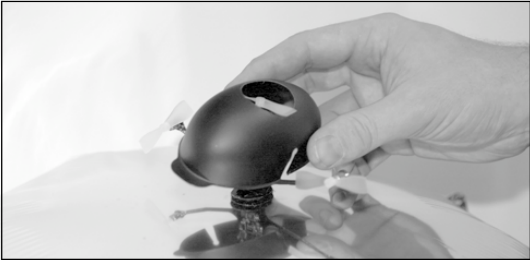
Fig. 5 - Slip the plastic dome over the central propeller, and align the slots with the motor arms, getting ready to attach to the balloon.
