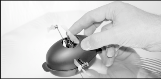
Fig. 6 - Ensure that the plastic dome is not touching the Microblimp Gondola circuit board, and get ready to use the self adhesive sticker “pockets”
