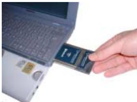
Insert the Bluetooth PC Card into a free PC Card slot
