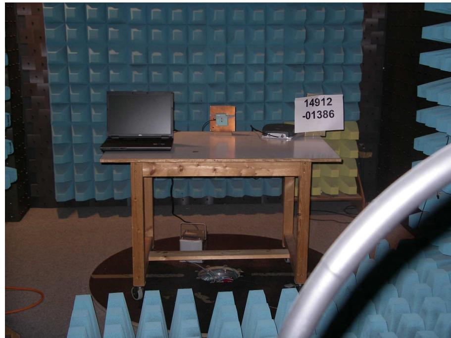
**Test setup for radiated emission measurement
