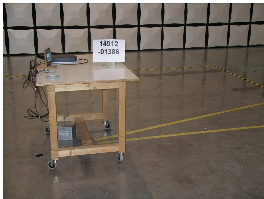
**Test setup for radiated emission measurement
