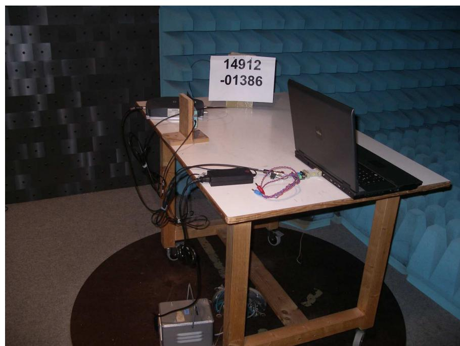
**Test setup for radiated emission measurement
