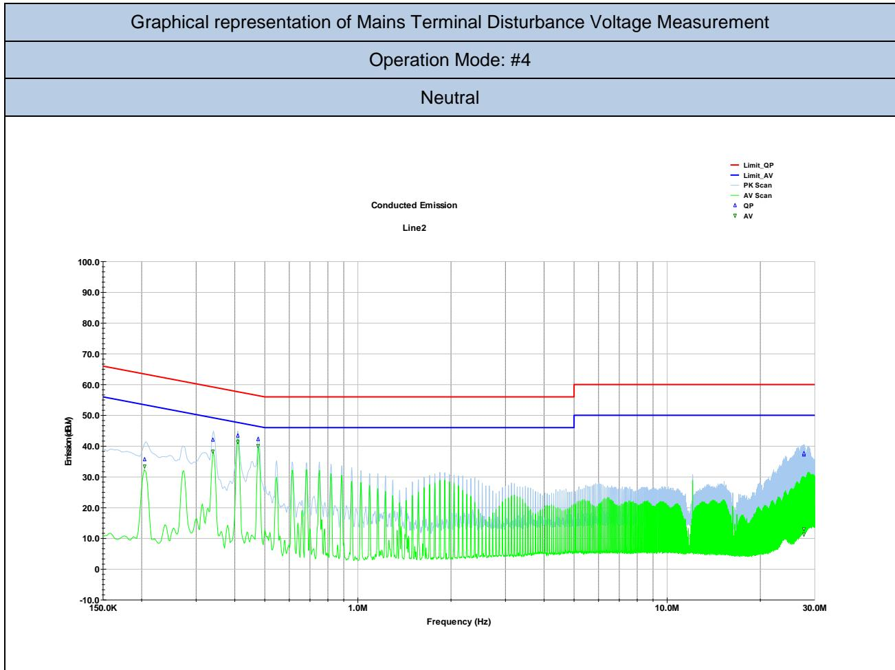
Final Measurement - Table representation of Mains Terminal Disturbance Voltage Measurement
