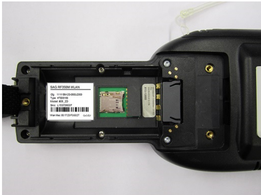
Picture 6. Simatic RF350M inside label location.
