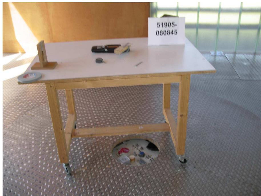
**Test setup for radiated emission measurement
