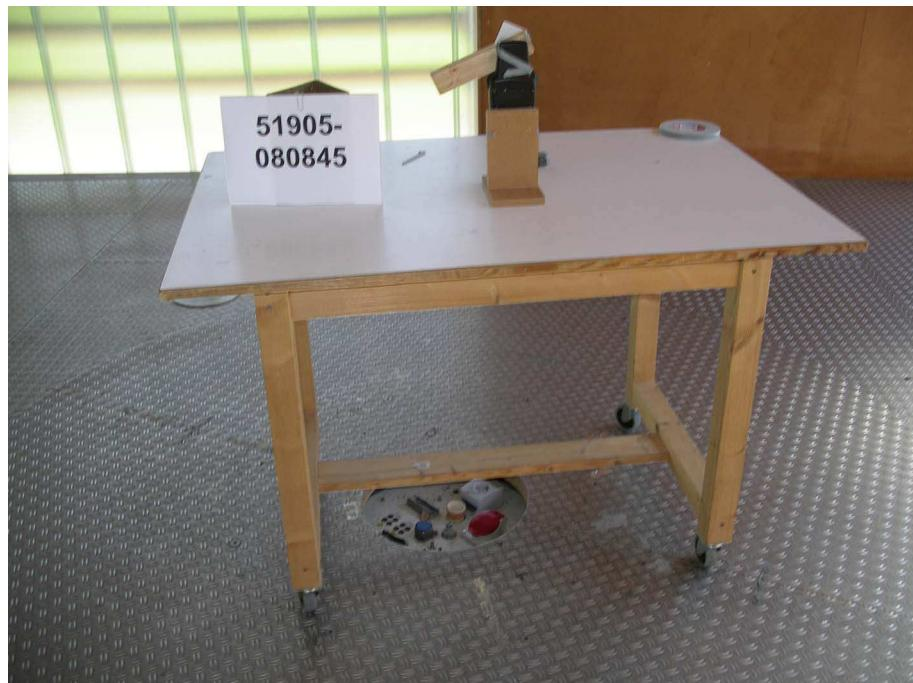
**Test setup for radiated emission measurement
