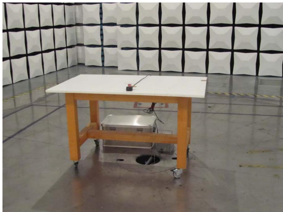
**Test setup for radiated emission measurement
