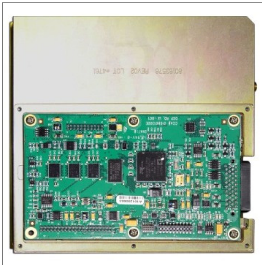
Photo 5 : VDR Module with Top Lid Removed Showing DSP Board
