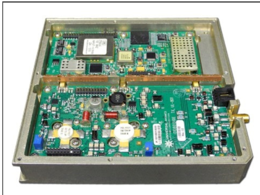
Photo 4 : VDR Module with Bottom Lid Removed Showing Mod-Demod Board (top) and Transmitter Board (bottom).
