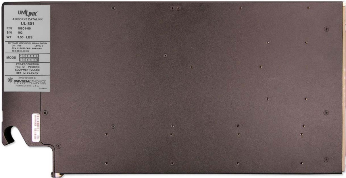
Figure 1 : UL-801 ID Label Location
