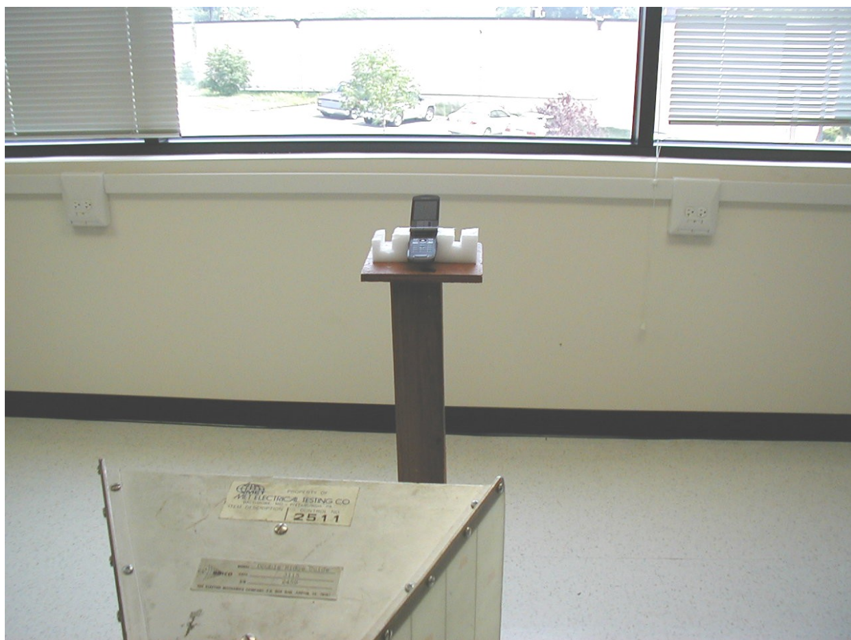
Photograph 1 EIRP measurement Setup
