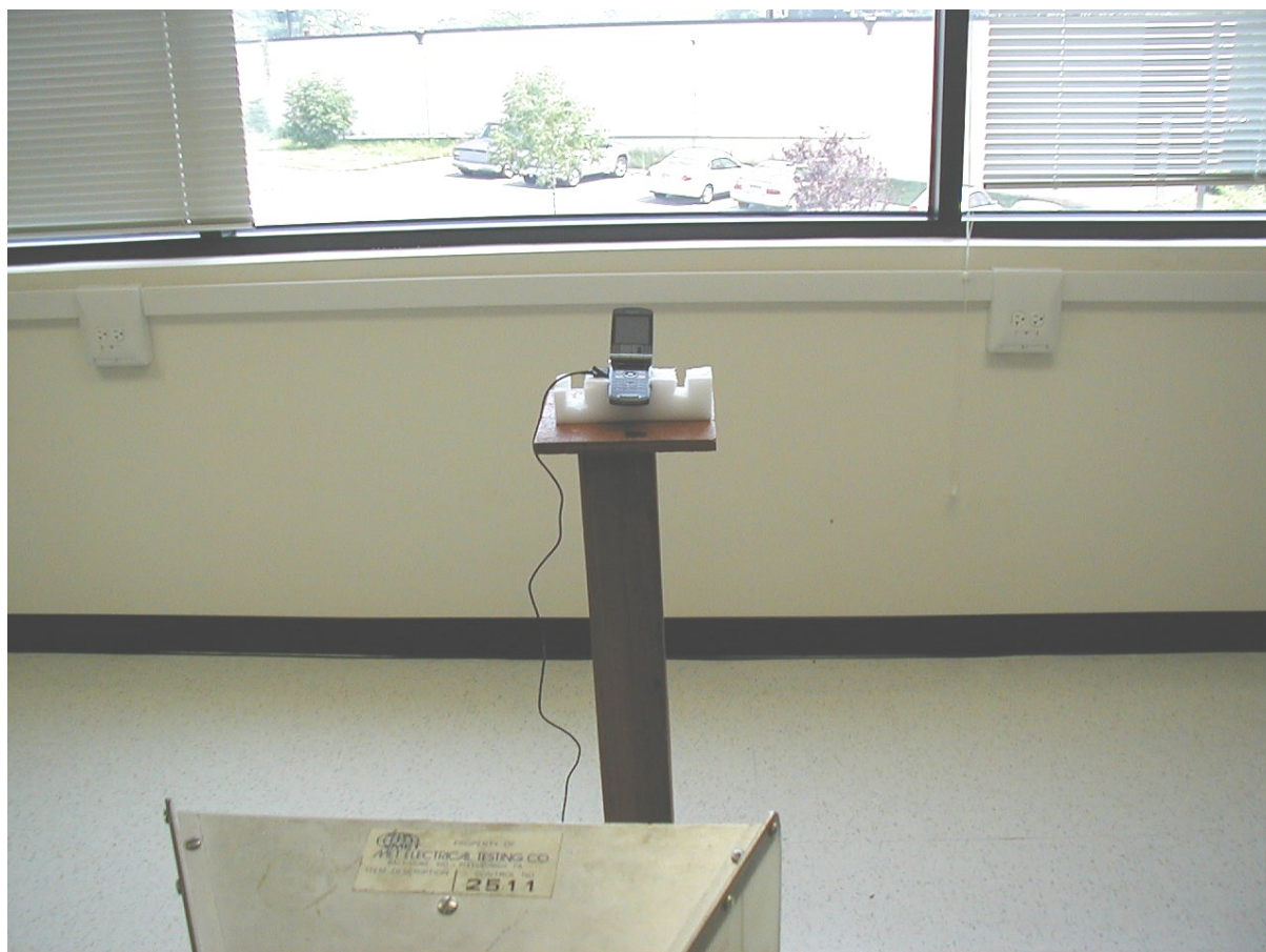
Photograph 6 Radiated emissions measurement Setup
