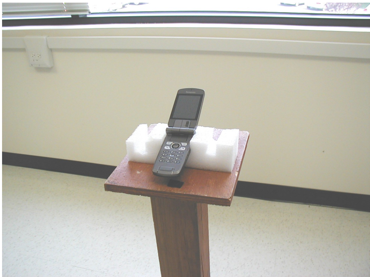
Photograph 2 EIRP measurement Setup
