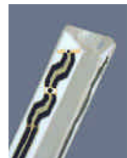
Figure 3.2 Probe Thick-Film Technique
