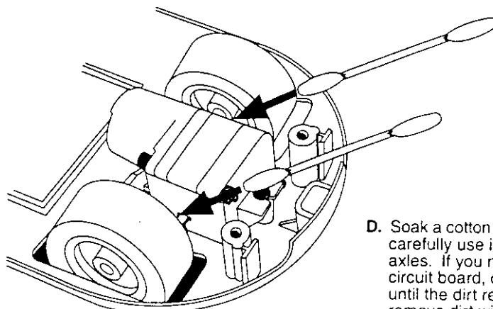
D. Soak a cotton swab in rubbing alcohol and carefully use it to clean the front wheel axles. If you notice dirt on the receiver circuit board, carefully blow on the board until the dirt releases. Do not attempt to remove dirt with any type of tool!
