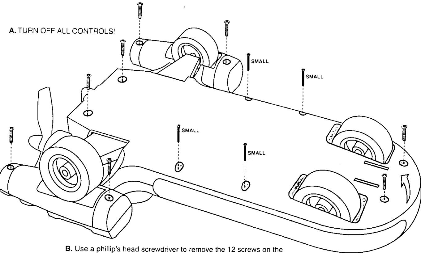
B. Use a phillip's head screwdriver to remove the 12 screws on the bottom of the landspeeder. (The diagram above will help you to put the screws in the correct holes once you have finished cleaning.)
