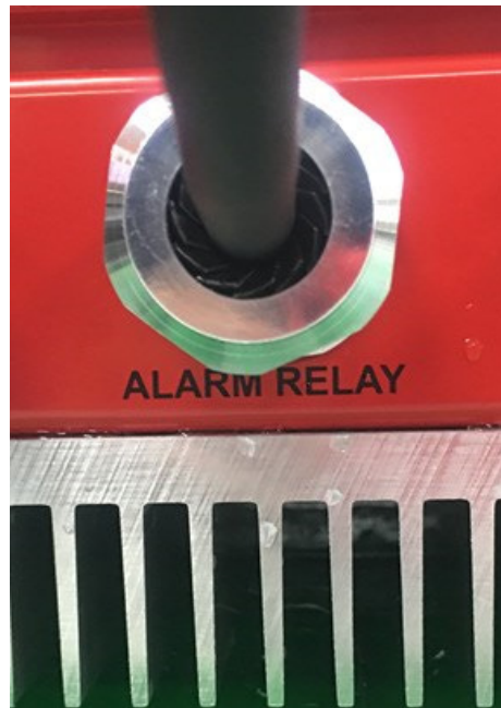
Figure 5-4: Alarm Relay 18-wire Gland Connector M6110
