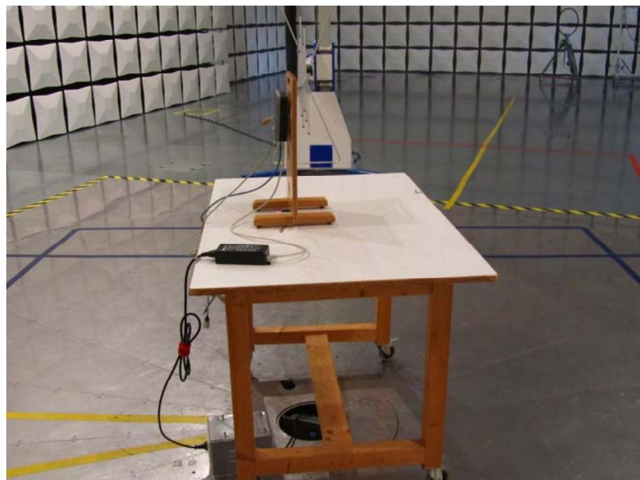
**Test setup for radiated emission measurement
