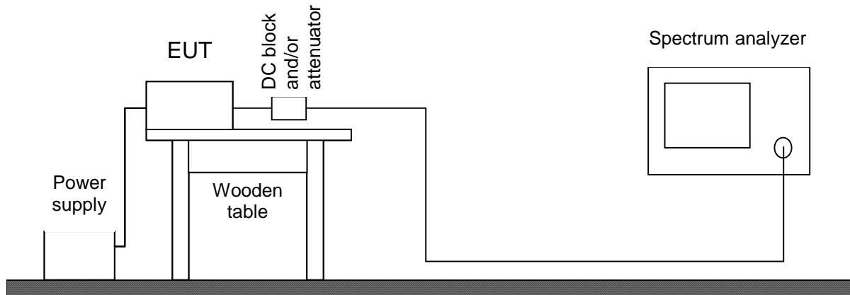
Test instruments used for conducted measurements:
