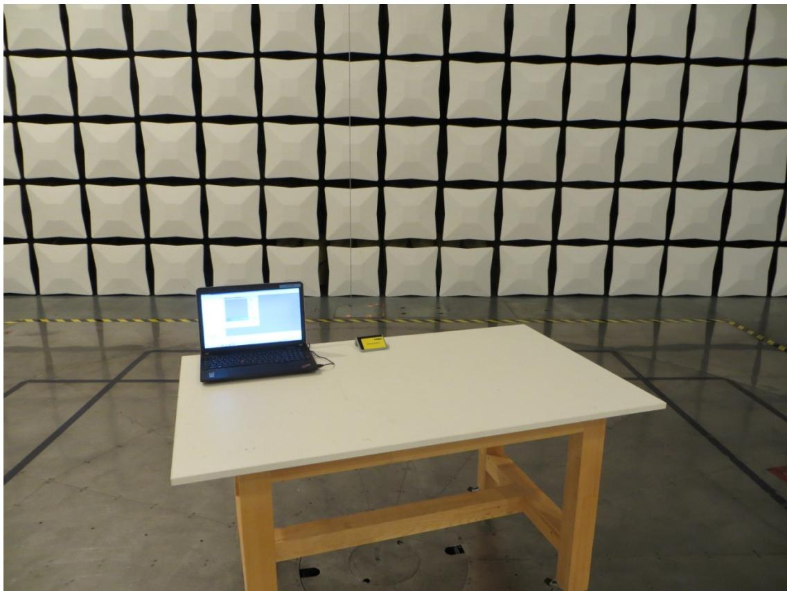
**Test setup for radiated emission measurement
