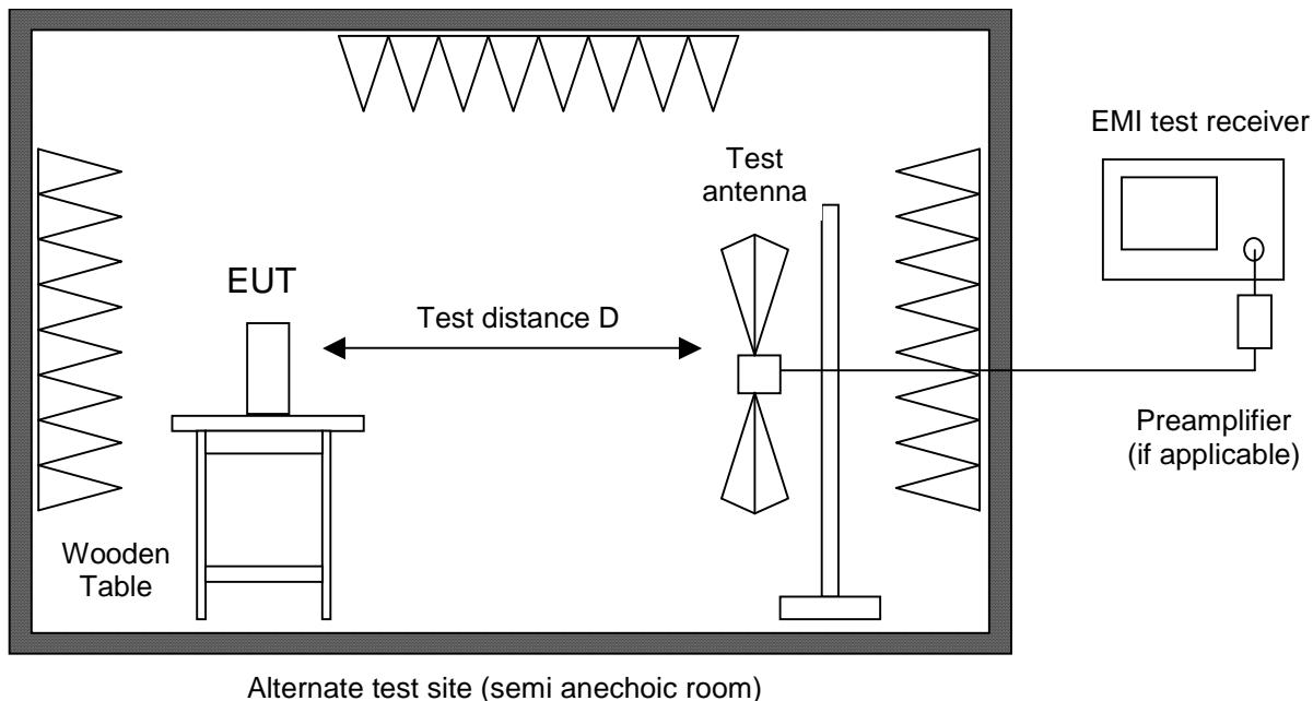
Alternate test site (semi anechoic room)
