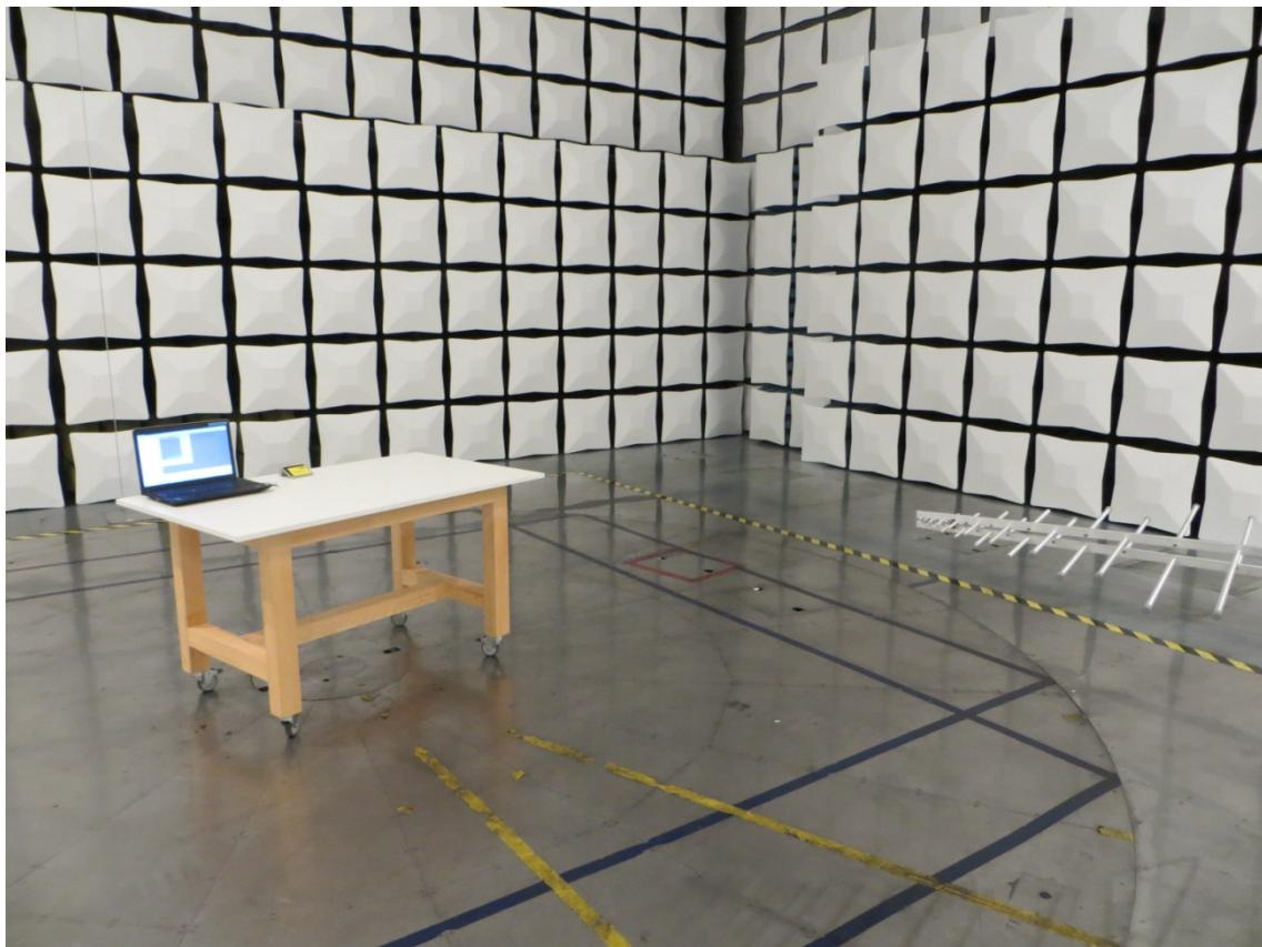
**Test setup for radiated emission measurement
