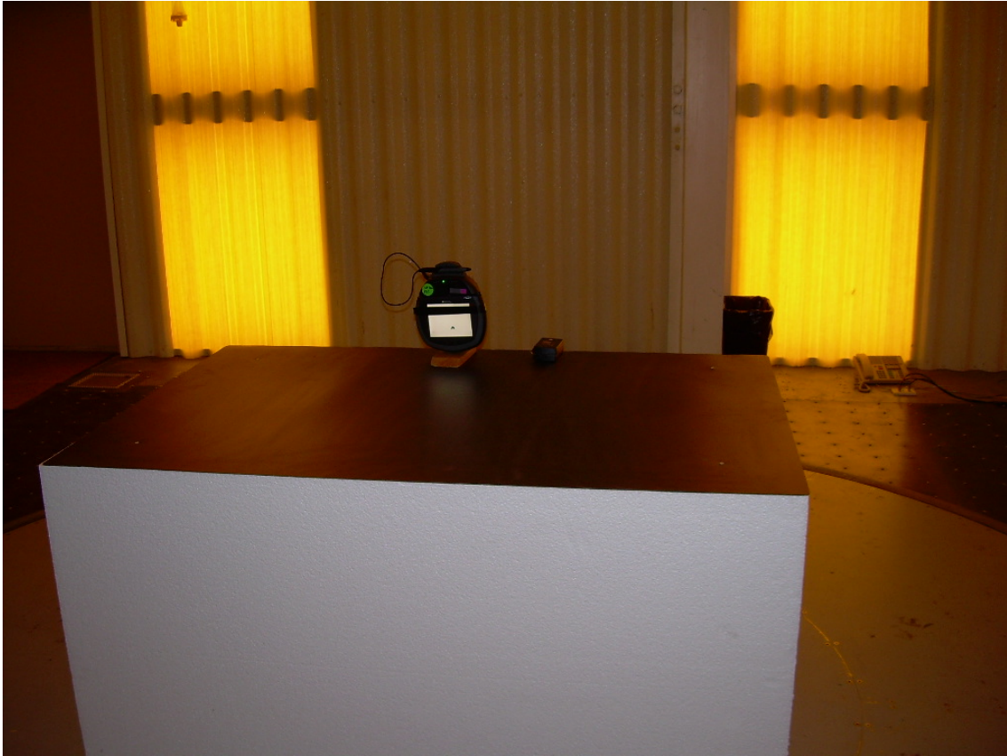
Front View Radiated Disturbance Worst Case Configuration
