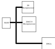
**ICE Control and Operation.** The brains of the ICE unit are a Zilog Z84C15 microprocessor. Located on a secure module with a 4Mbit memory chip, the microprocessor is used to control all functionality and operation of the ICE unit. A Xilinx FPGA chip is used to reduce glue logic and for control registers needed to control internal and external peripherals. A Zilog Z8 microprocessor can be utilized if additional security is needed.
