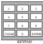
**KEYPAD.** The keypad on the ICE unit consists of ten numeric keys ( 0 through 9) and two special function keys. The special function keys are “CLEAR” and “ENTER”. Additional soft keys can be created using the touch screen display and software code. The OS code for the ICE unit continually scans the keypad for a key press during normal operation.
