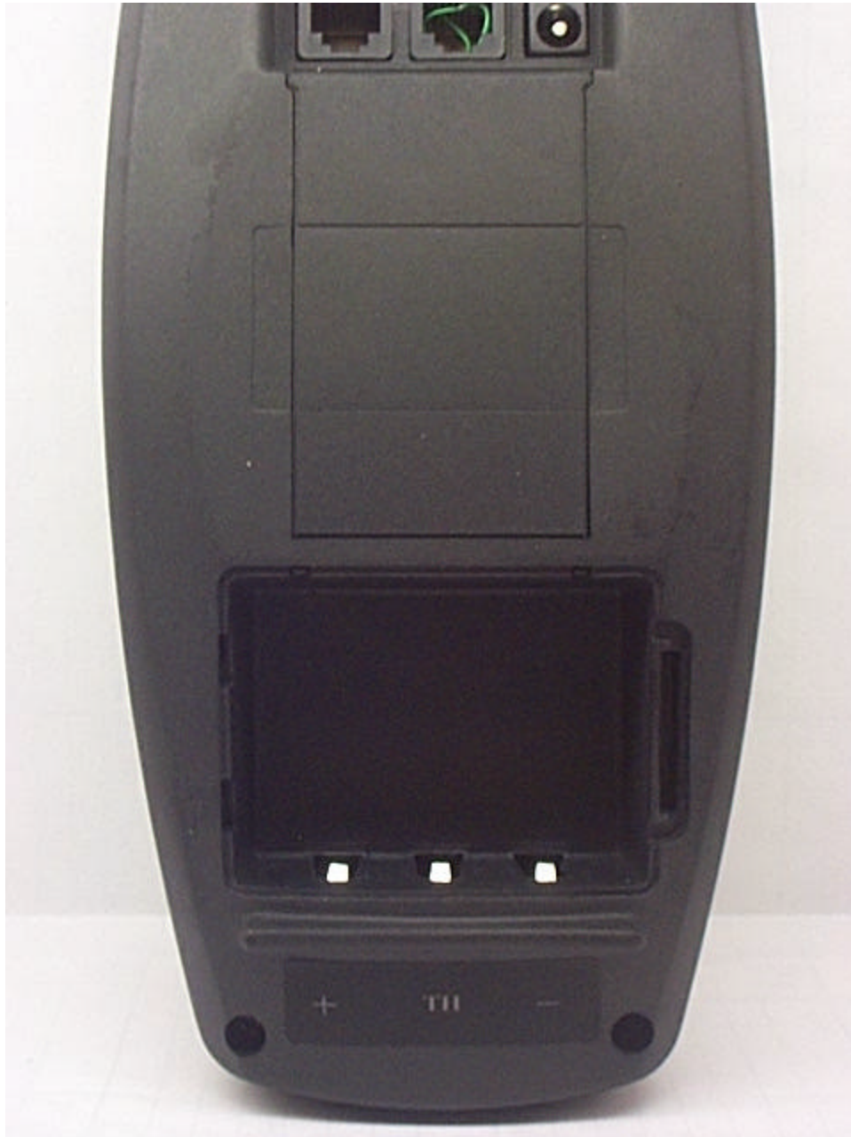
Hypercom Point of Sale Device SmartICE with a Novatel NRM-6832 transmitter CDPD: Back, battery compartment
