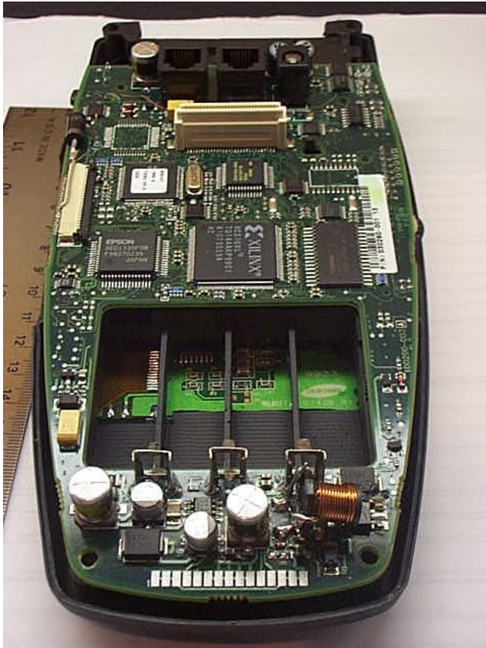
Hypercom Point of Sale Device, SmartICE with RIM R902M-2-0 Transmitter, Mobitex:Back open, board connected to transmitter detail
