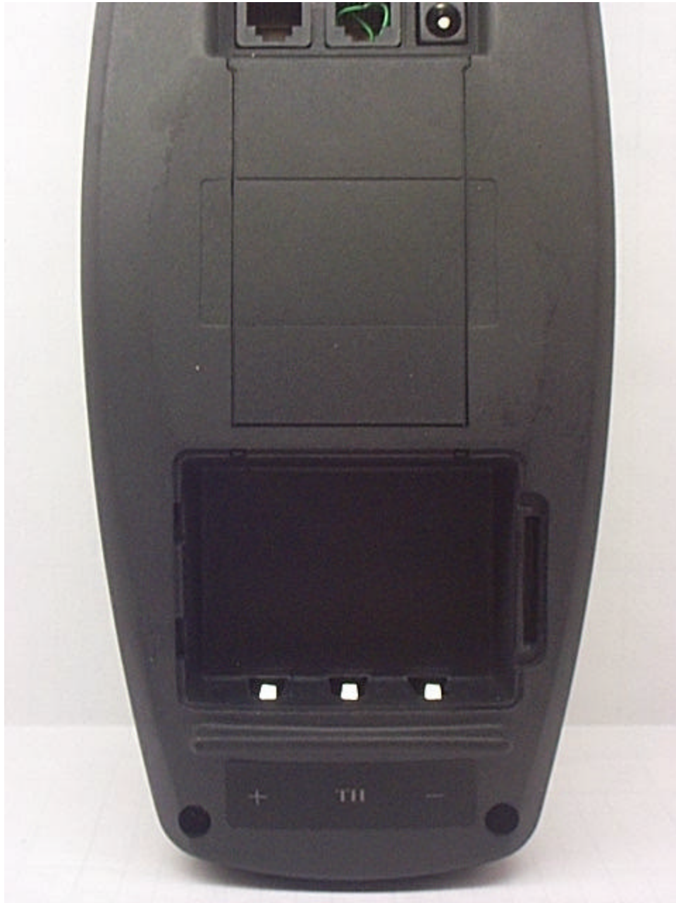
Hypercom Point of Sale Device, SmartICE with RIM R902M-2-0 Transmitter, Mobitex:Back, battery compartment
