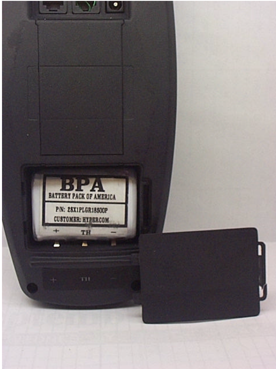
Hypercom Point of Sale Device, SmartICE with RIM R902M-2-0 Transmitter, Mobitex:Back, battery
