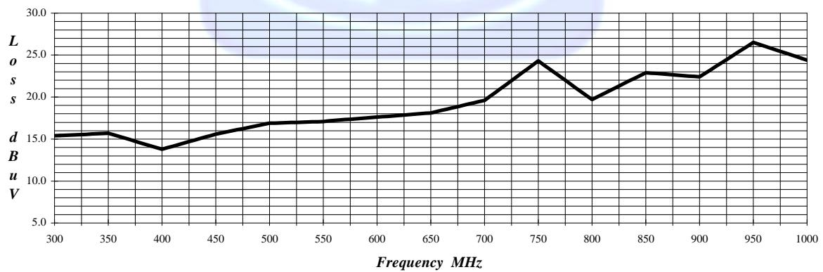
**PREAMPLIFIER EFFECTIVE GAIN AT 3 METERS PA-102 S/N: 1017 Lab "D"
