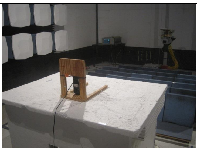
Test setup at 3 meter distance (>1 GHz) - Rear
