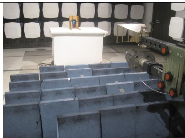
Test setup at 3 meter distance (>18 GHz) - Front
