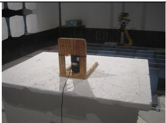
Test setup at 3 meter distance (>18 GHz) - Rear
