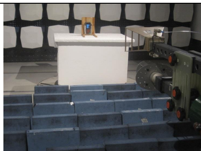
Test setup at 3 meter distance (>1 GHz) - Front
