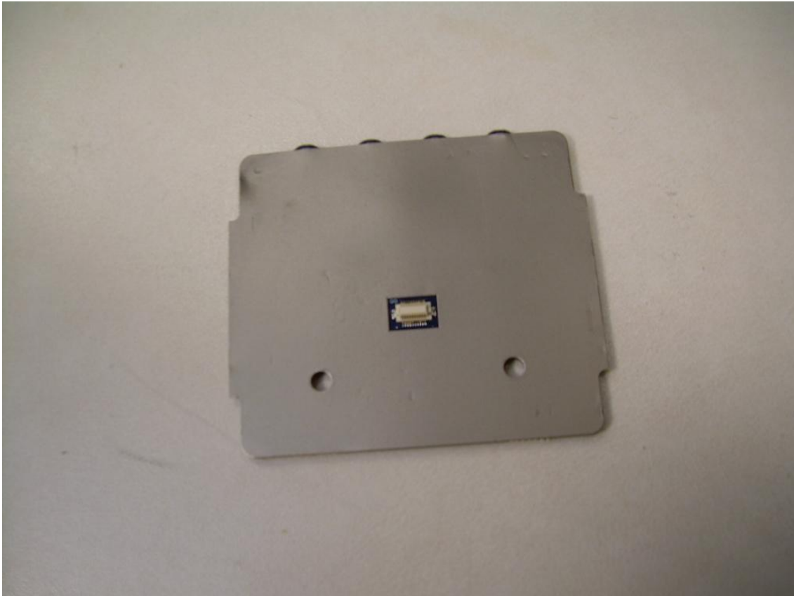
Back Side of the RF PCB with RF Isolation in Place
