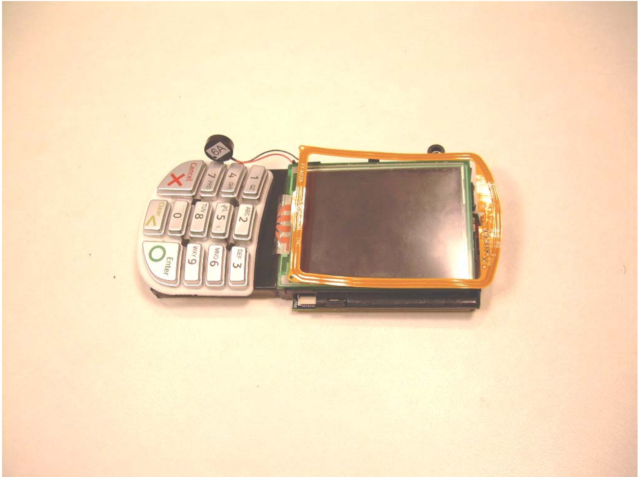
Photograph 22 - Top View of the Keypad/Display Unit
