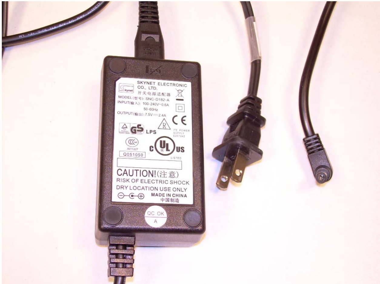
Photograph 31 - View of the Dock/Charger Power Supply
