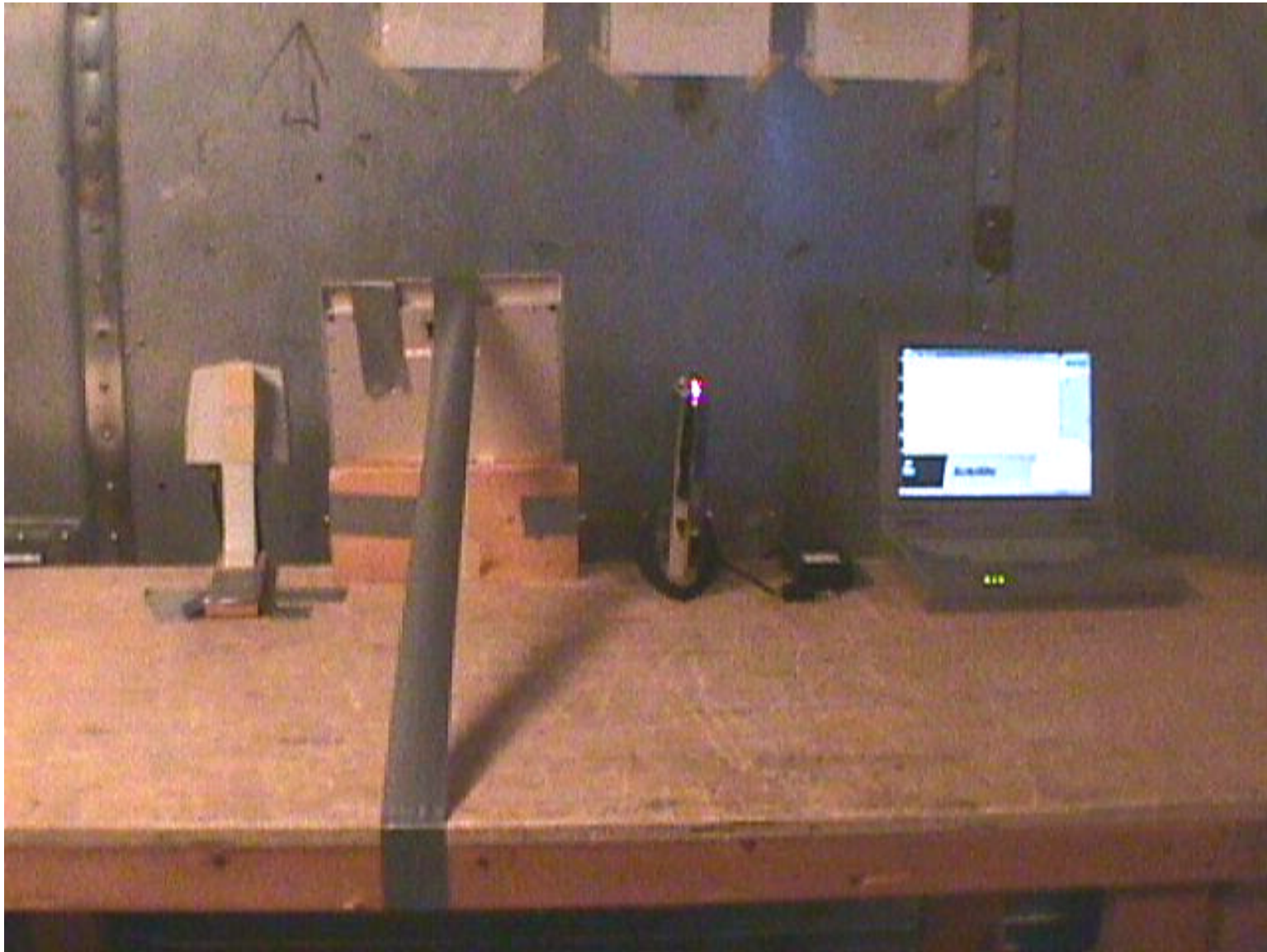
Test setup for AC Power-line Conducted Emissions in a Shielded Chamber (Front View)
