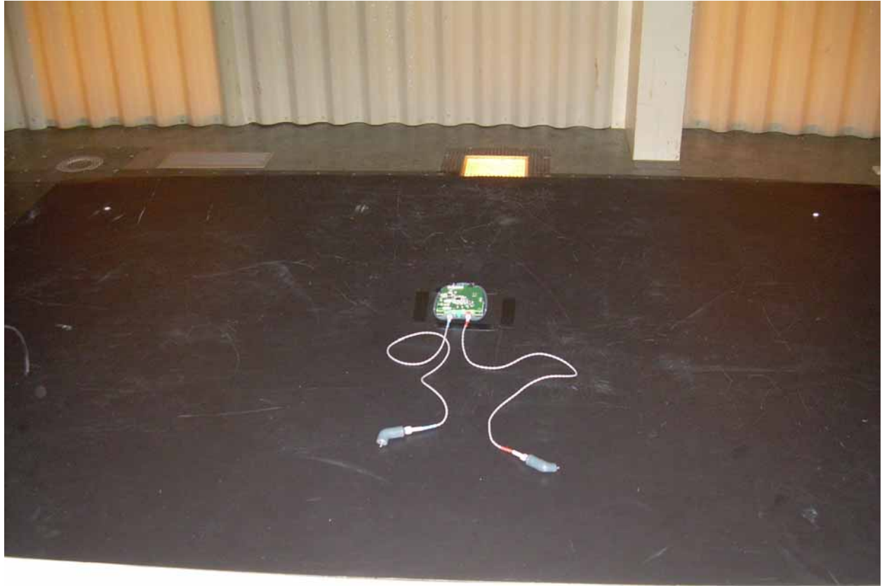
Photograph 1 - View Radiated Spurious Emissions in the Restricted Bands - Horizontal Placement
