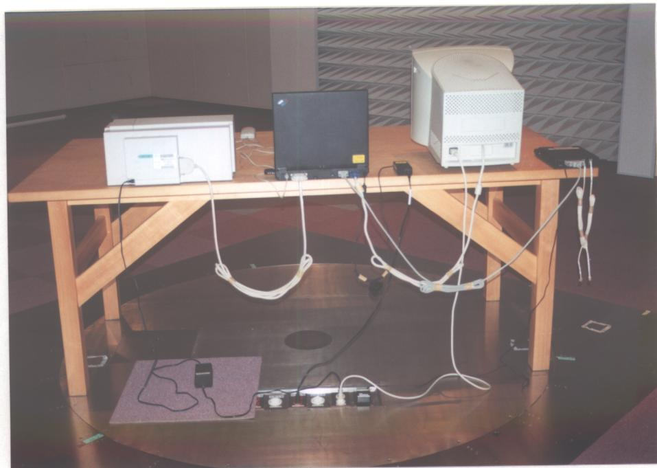
This cable routing was attempted to maximize the radiate emission.
